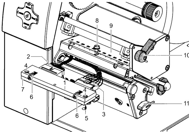
**Fig. 18:** Removing and installing the printhead
