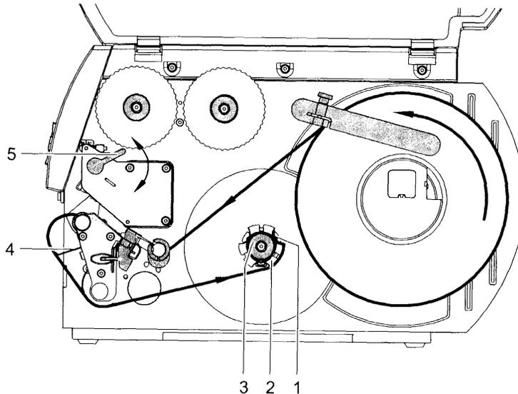
**Fig. 7:** Guiding the label strip in Rewind mode
