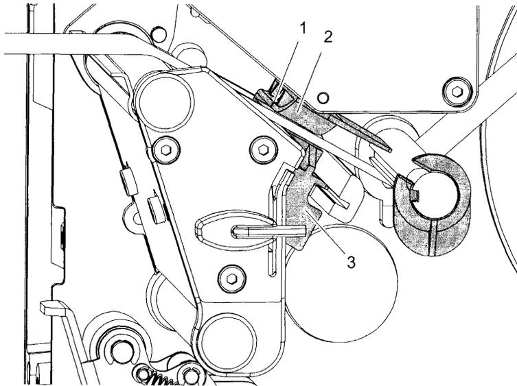
**Fig. 6:** Setting the label sensor
