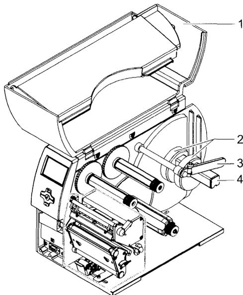
Fig. 4: Installing the core adapter
