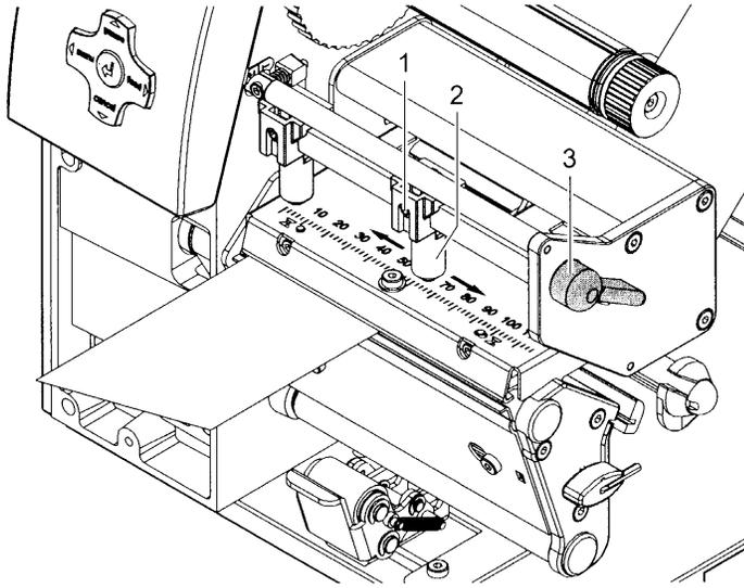
**Fig. 9:** Setting the head locking system
