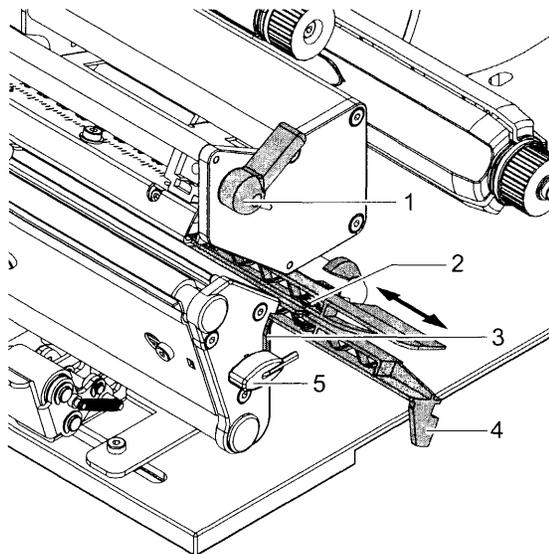
1. Turn lever (1) counterclockwise to lift the printhead.
