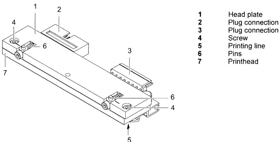
Fig. 17: Structure of the printhead
