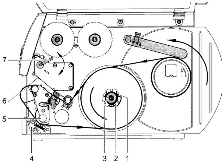
**Fig. 10:** Removing the wound roll
