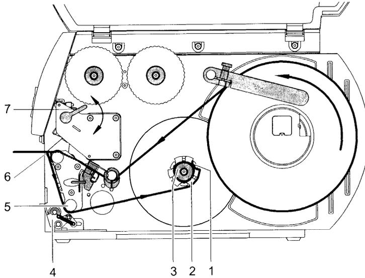
**Fig. 8:** Guidance of the liner in Peel-Off mode
